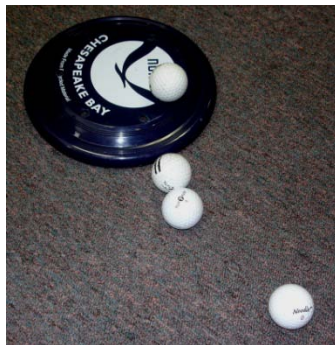
Figure 8, Payload Failure from rolling out.
