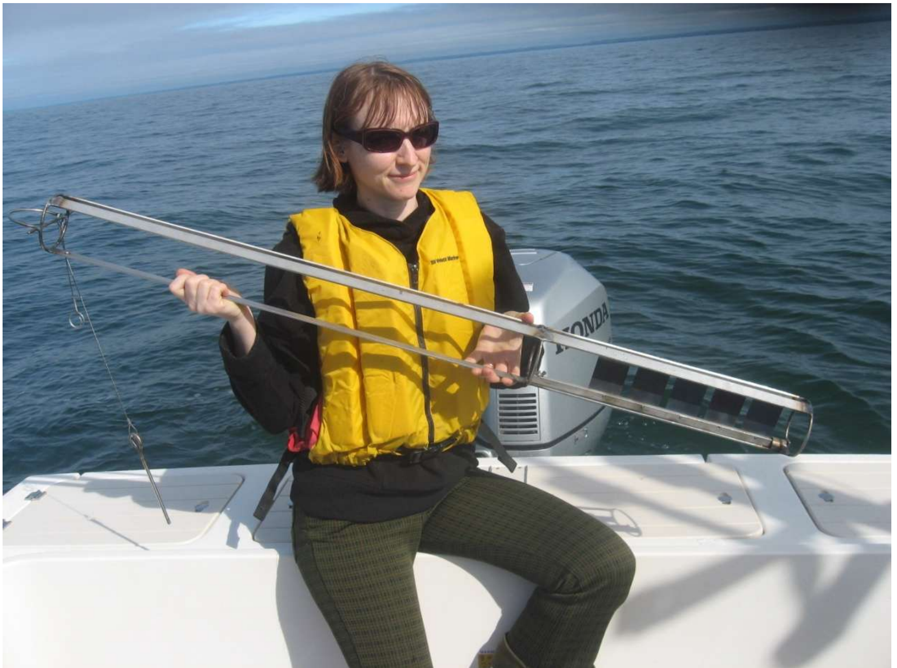
Graduate Student Joanne Elmoznino holding the LISICOS passive sampling device.
