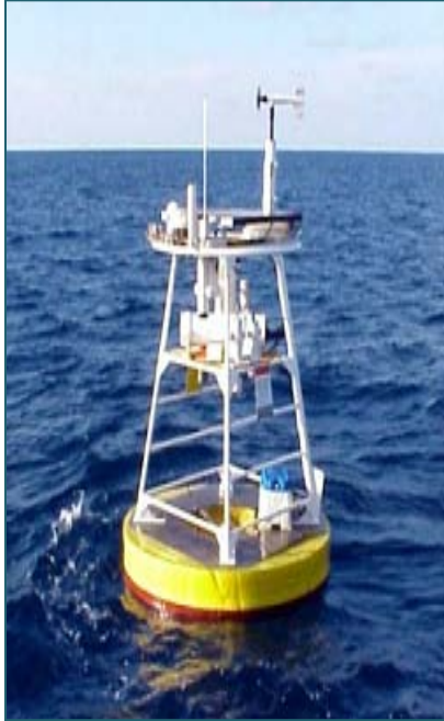
The Coastal Ocean Monitoring and Prediction System (COMPS) for West Florida provides data needed for a variety of management issues, including more accurate predictions of coastal flooding by storm surge, safety and efficiency of marine navigation, search and rescue efforts, and fisheries management, as well as supporting basic research. COMPS sites are operated in close collaboration with Florida local and state emergency management officials. Wherever possible, there are direct line-of-sight radio links from the observing site to the local emergency operations center. COMPS personnel provide training for the emergency managers on how to access and use the data from each site. Photo: Cliff Merz, USF/St. Petersburg
