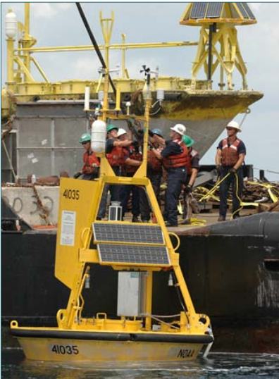
The USCG ELM deploys a UNCW/US Marine Corps weather and oceanographic buoy 5 miles offshore of the Camp Lejeune Marine Corps Base. The buoy will provide valuable data for boaters and mariners and play a significant role in Base training and operations.
