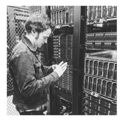
~5,000 processor cores ~1.5 petabytes of functional storage/5 petabytes of actual storage (~1,500 hard drives) Level 2 Fat Tree Infiniband Network, 40 Gb/Sec node to node). 240 Gb/Sec cluster to cluster
