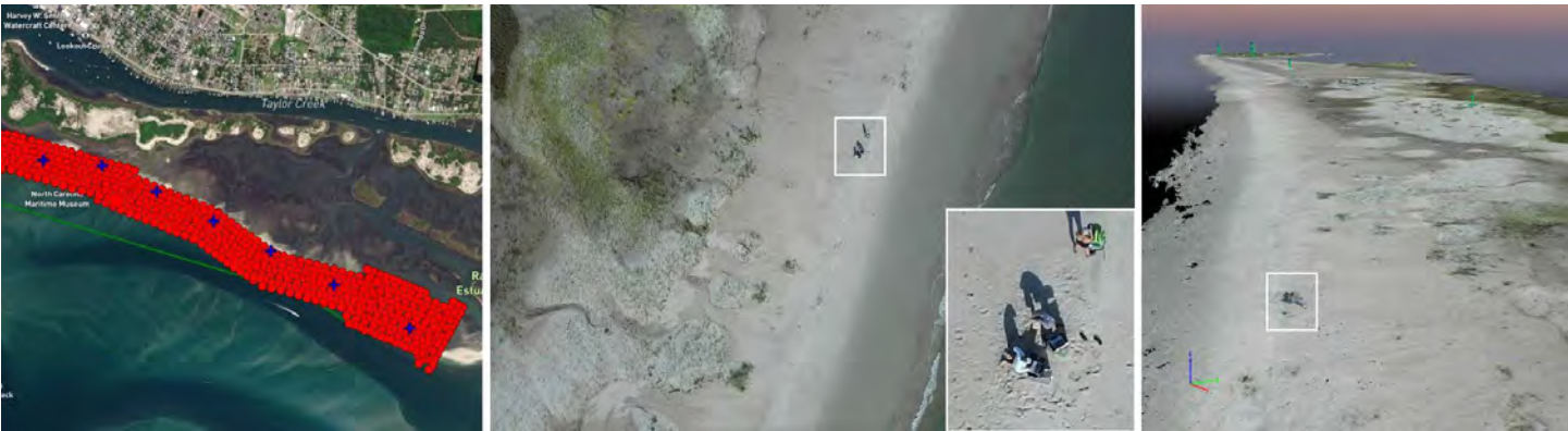
Figure 1. From mission to point cloud. Left Panel: Image locations (red dots) over Bird Shoal (Rachel Carson Reserve, North Carolina National Estuarine Research Reserve) flown with a senseFly™ eBee Plus equipped with senseFly™ S.O.D.A. camera. Center Panel: Image taken over the remote pilot crew with close up in the inset. Right Panel: Resulting point cloud from the image dataset processed through Pix4D Structure from Motion software with the same reference boxed at an oblique view. Photos: Duke Marine Robotics and Remote Sensing (MaRRS) Laboratory
