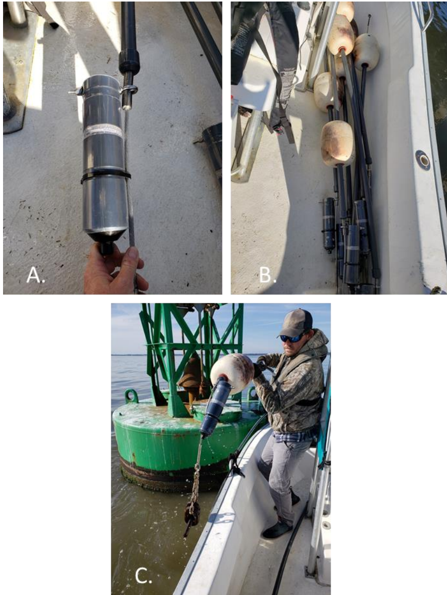
Figure 2. A. VR2W attached to mooring cable; B. Receiver moorings prior to deployment; C. Receiver retrieval.
