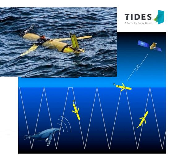
Integrate and test near real-time passive acoustic monitoring capability on SkIO glider
