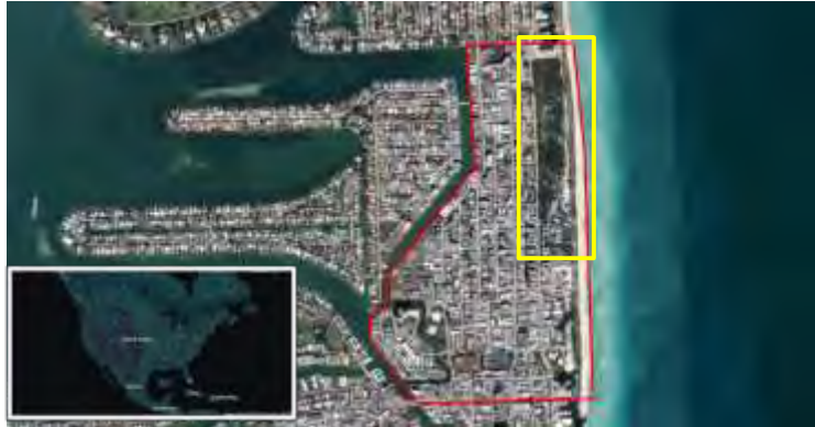
In red, photogrammetry area. In yellow, Lidar area. Target area was 410 acres. Census Tracts: 12086003909, 12086003911, 12086003913
