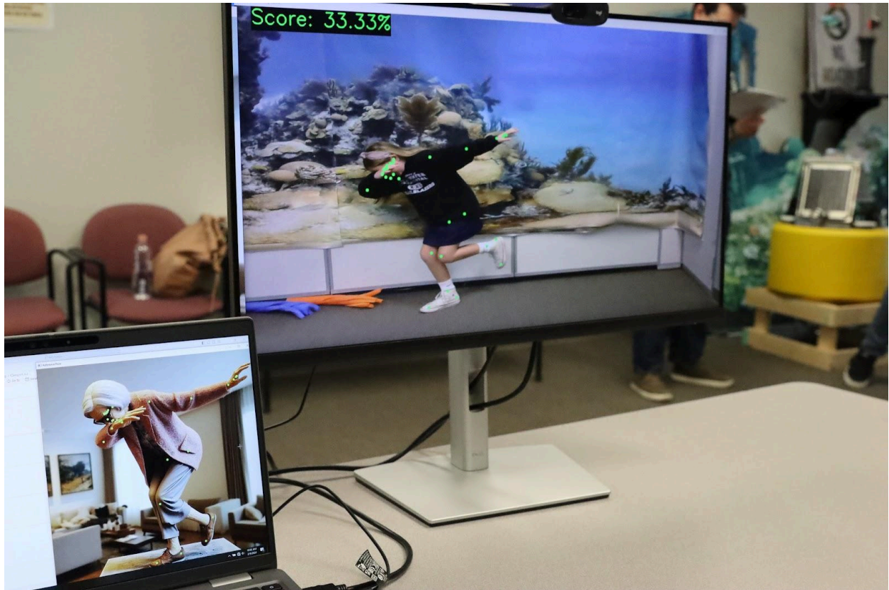
Figure 4. Demonstration of the pose detection and matching activity as powered by the Google Pose detection module. Students were scored on their ability to match the pose of a reference image. In the photo above, the student only scored a 33% on their ability to match the reference image of a grandma performing 'the dab.' Photo Credit: Carol Davis, FWRI.
