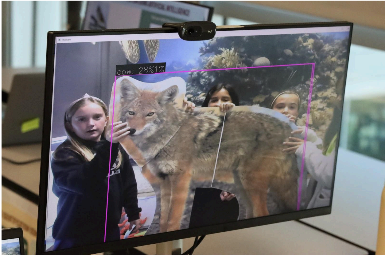
Figure 2. Demonstration of the animal detector and classifier activity. Students held up large cutouts of pieces of animals in front of a webcam, where the YOLOv8 classifier would draw a bounding box and attempt to identify the animal. Here, students held up the three pieces of a coyote, which was incorrectly identified as a cow. Usually, the module could correctly recognize the coyote with relatively high confidence. Photo Credit: Carol Davis, FWRI.
