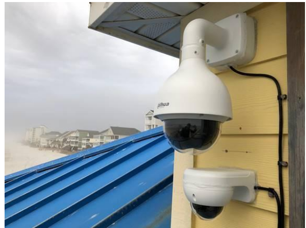
Image 2: Pictured above is an example of a shore-based web camera. (Credit: Surfline)
