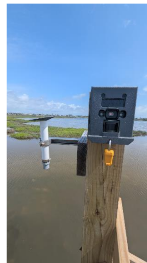
Low-cost water level sensor (Hohonu) installed near flood prone road with camera (Reconyx Hyperfire HF4K)
