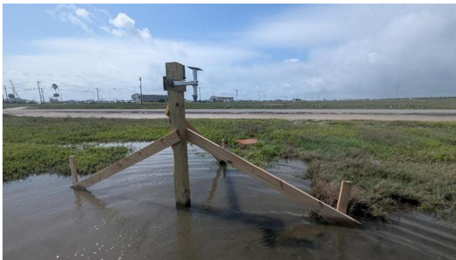
Low-cost water level sensor (Hohonu) installed near flood prone road with camera (Reconyx Hyperfire HF4K)
