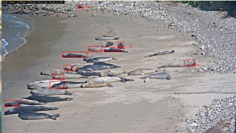
Missed detections due to lack of contrast(lighting) or change in distance or view angle
