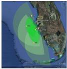
A comprehensive coastal ocean observing and modeling system is maintained by USF, including *in-situ* moorings, overlapping high-frequency (HF) radar arrays, occasional glider transects and models that downscale from the deep-ocean, across the shelf and into the estuaries.
